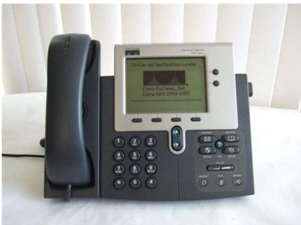
2 LCD screen Displays features such as the time, date, your pho Also controls the ringer volume if the handset is in its cradle, and the LCD screen contrast. For more information on adjusting the
